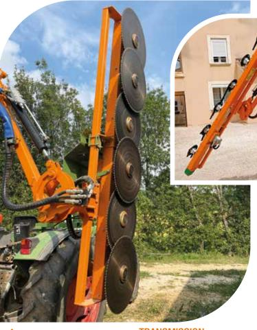
2 TYPES OF CUTTING TOOLS cutting discs or saw blades
